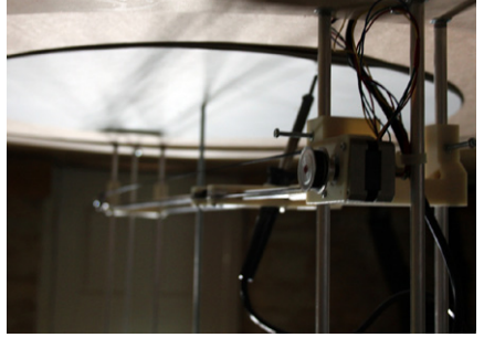
Looking down over the Climate Machine as it burns carbon dioxide levels from 1959 as a circular graph onto paper
